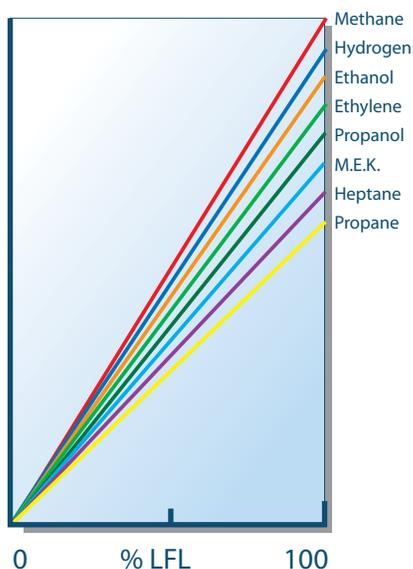
Catalytic sensors will exhibit considerable response drift when exposed to constant levels of flammable vapors. There is no way to ensure that they are responding accurately—or even responding at all—other than by injecting a known concentration of test gas through the flame arrestor. This calibration test should be done frequently, as this type of sensor gives no notice of failure.
