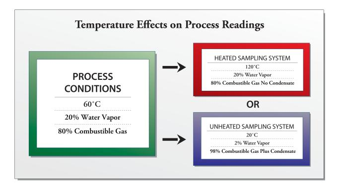
Keeping all parts of the sampling system and analyzer at 250°F (120°C) prevents this error under most conditions. Also, a heated analyzer prevents condensation of heavier, less volatile hydrocarbons. Keeping all sample-wetted parts of the sampling system and analyzer at a high temperature will ensure that these combustible vapors are properly measured.
