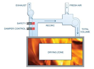
Otherwise, a fixed damper must be set so that solvent vapor concentration input cannot exceed 50% LFL (for the highest design solvent).
