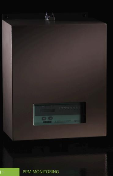
Control Instruments' flame ionization detectors are industrial grade analyzers that measure the emissions of total hydrocarbons and VOC's in the parts per million range. The Model SNR650 is a high temperature unit that mounts directly onto the process ductwork, eliminating sample handling problems and resulting in fast and easy installation, low maintenance, less downtime and very fast total system response.
